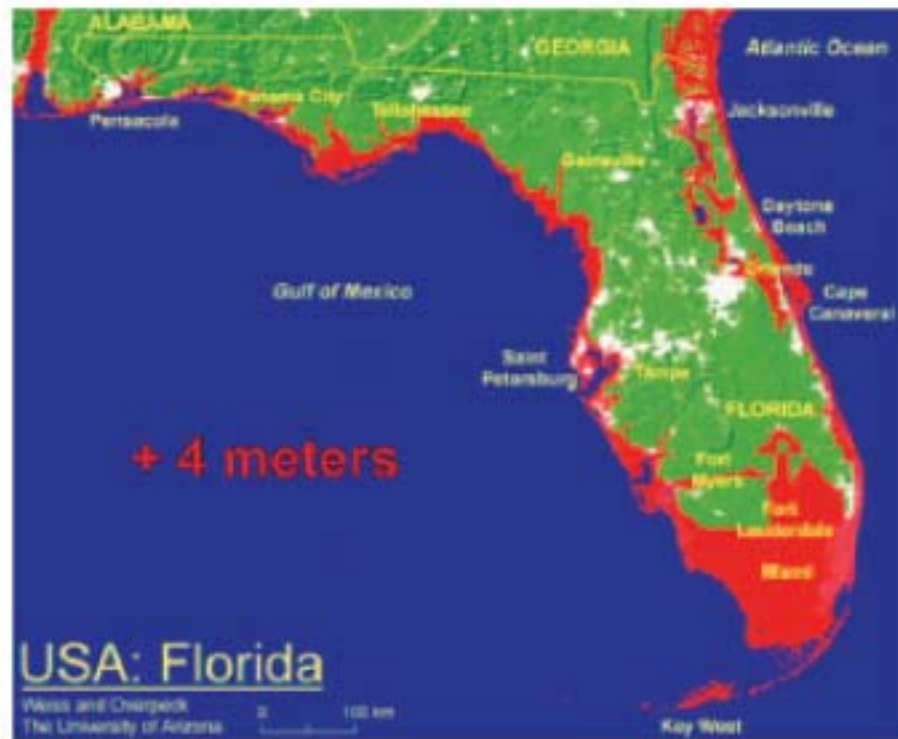
Figure 12. Coastal inundation arising from increases in sea level. Includes only the effect of the thermal expansion of warming ocean waters. Excludes sea-level changes due to melting continental ice sheets.
